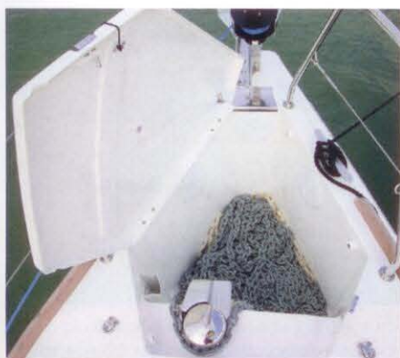
A deep anchor locker, formed as part of the deck moulding, houses the rode and windlass
