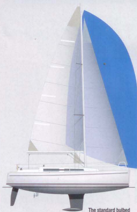
The standard bulbed fin gives a draught of 1.9m (6ft 3in)
