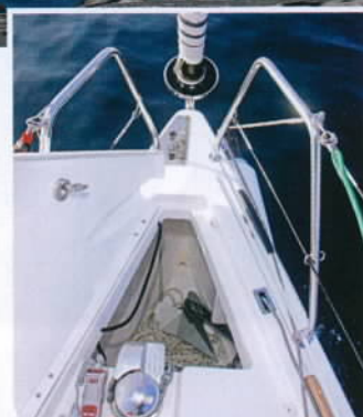
The anchor locker, big enough to take our Delta, has a windlass
